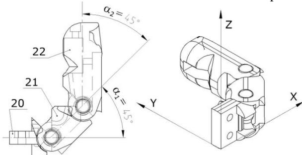
Fig. 6. Location and orientation for printing of a finger.
