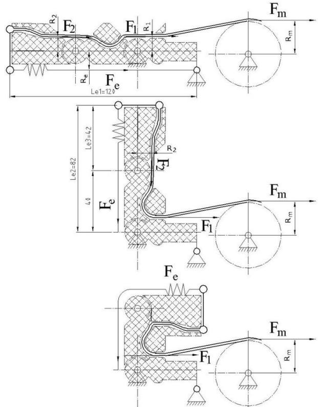
Fig. 7. Stages in the fingers movement and location of the forces.
