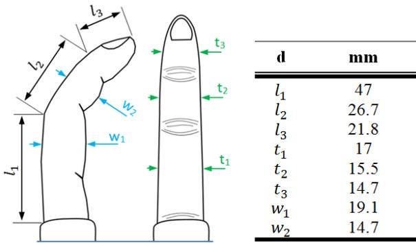
Fig.1. Dimensions of a human finger [3].
