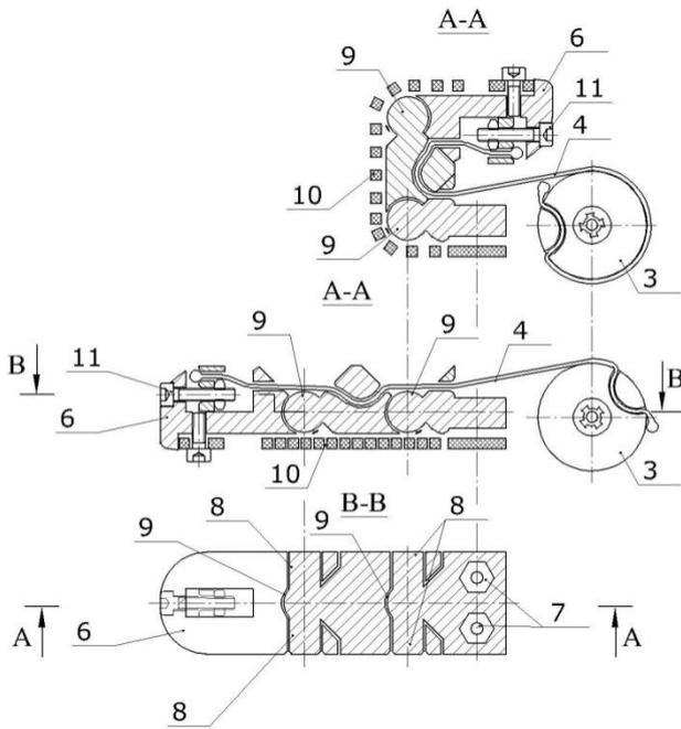
Fig.4. Structure of the hand's fingers.
