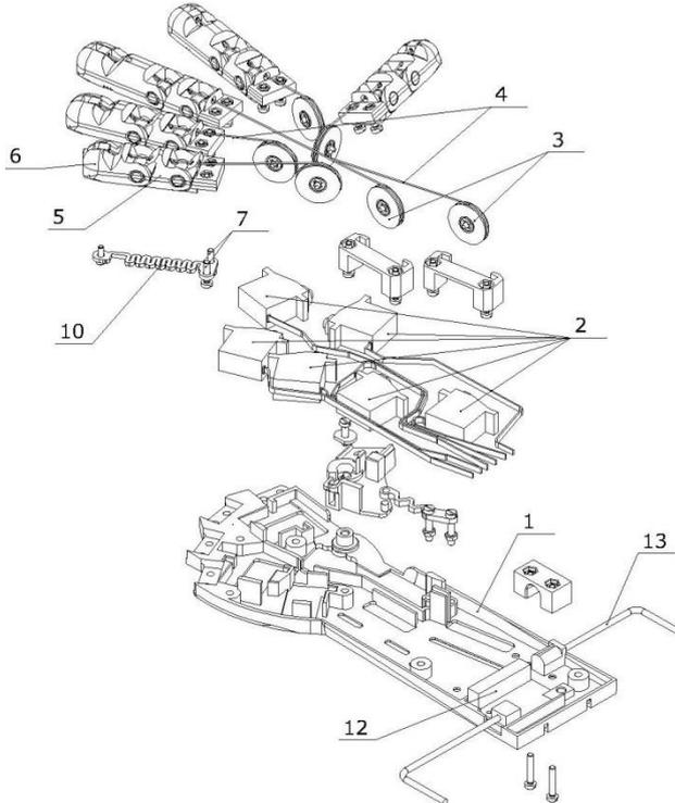
Fig. 2. Basic components of the hand.
