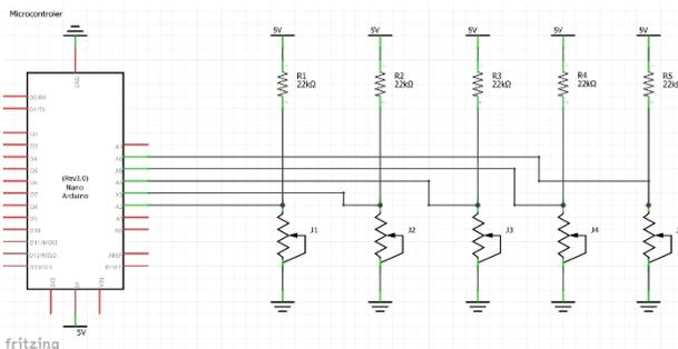
Fig.9.An electrical scheme of the glove.
