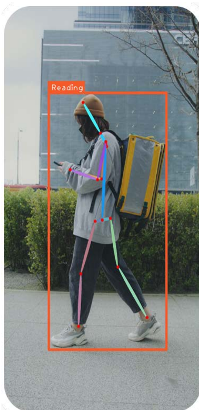
Fig. 2. Machine vision recognizing human and its limbs
