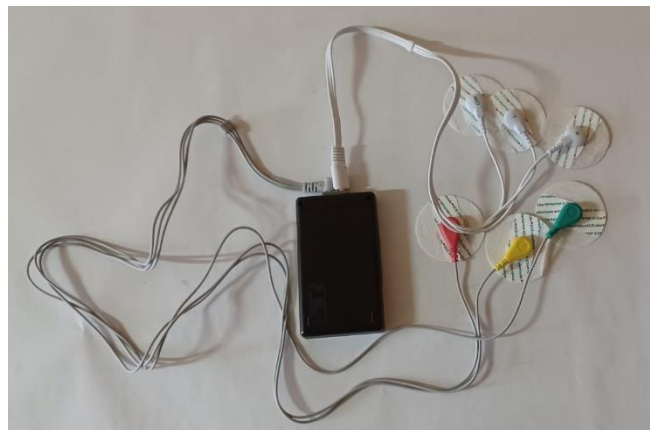
Fig.6 prototype of the ADS1293 based autonomous wireless ECG monitor
