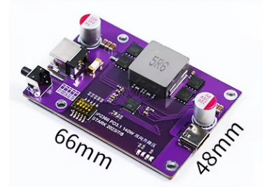
Fig. 5. USB PD controller IP2366
