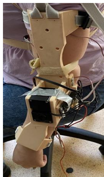
Fig. 7. Photo of the orthosis attached to the shoulder girdle
