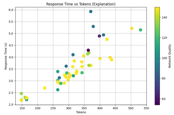
Fig. 5 Relationship between the API response time (in seconds) and the number of tokens received according to the network congestion for question explanation
