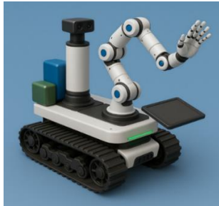
Fig.6 3D image of a variant of a mobility mechanism with a chain for a cobot.
