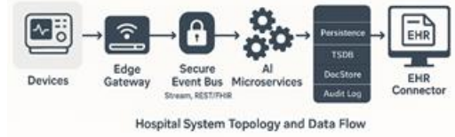
Fig. 2 — System Topology and Data Flow (Edge → Bus → Core → EHR)
