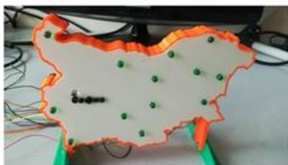
Figure 3: Interactive 3D-printed map of Bulgaria equipped with LEDs positioned at major city locations.
